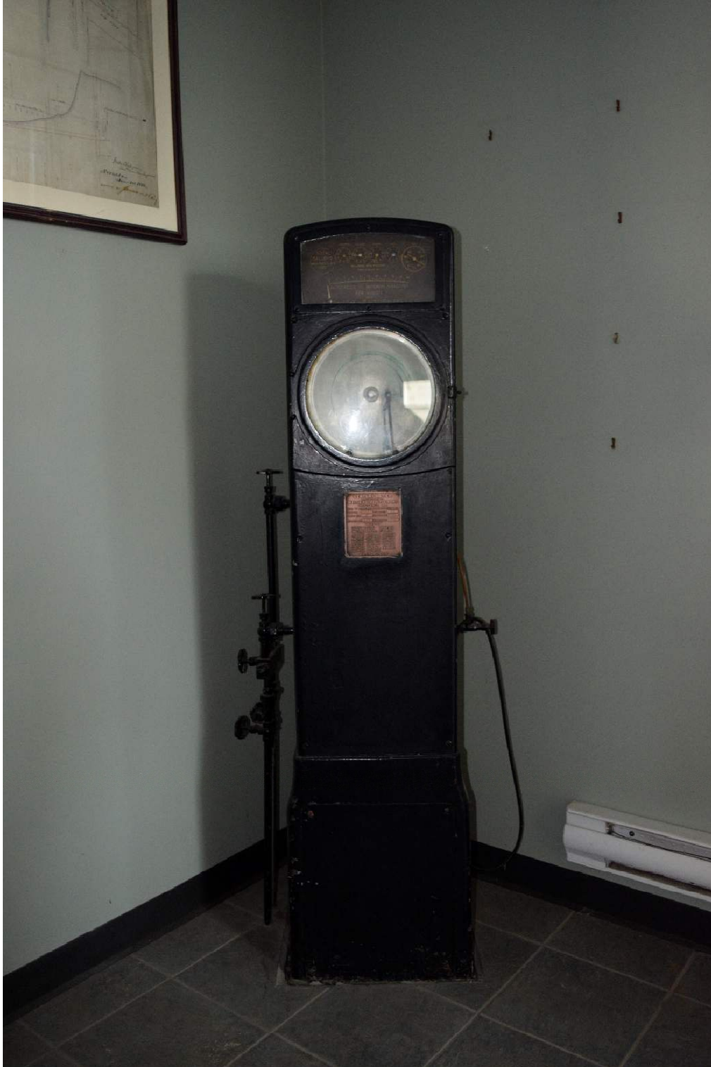
FIGURE 43: ORIGINAL VENTURI FLOW METER IN NORTHWEST CORNER OF OFFICE
